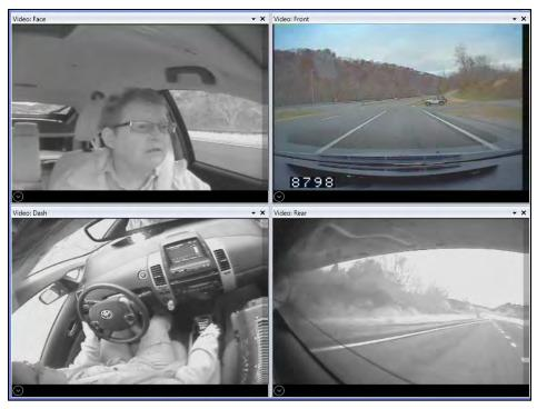
Figure 1. Multiplexed image of the four camera views. Top left: view of the driver's face. Top right: view of the forward roadway. Bottom left: over-the-shoulder view of the driver. Bottom right: view of the rearward roadway. (Note: Driver shown is a VTTI researcher.)
